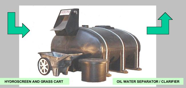
Dirty water is pumped from the primary sump to the solids separation hydroscreen. Grass trash and dirt are filtered by the screen and collected in a dump cart. Filtered water is then discharged to the combination oil-water separator / clarifier where free hydrocarbons and fine solids are removed. Settled solids are dewatered in a sludge dewatering drum.
